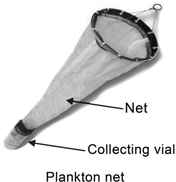
Fig. 3. A simple plankton net for collection of plankton from surface water.
