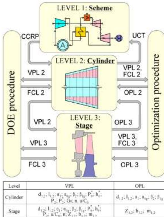
Figure 7.9 The structure of optimal design technique.
