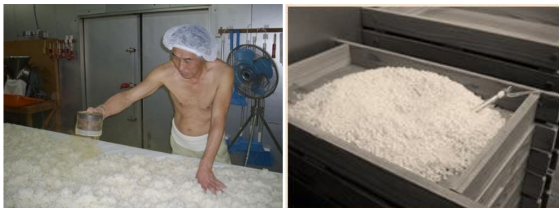
Fig. 7.3 Preparation of koji in sake production process.
